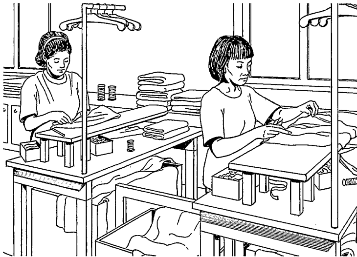
Figure 8: Double height work tables can be very practical for trimming and finishing tasks
