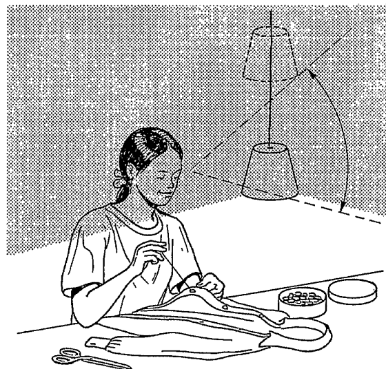
Figure 4: A shaded lamp should be placed at the appropriate height
