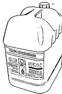
Figure 8: Containers with solvents should be clearly labelled. Workers should be informed when using dangerous solvents
