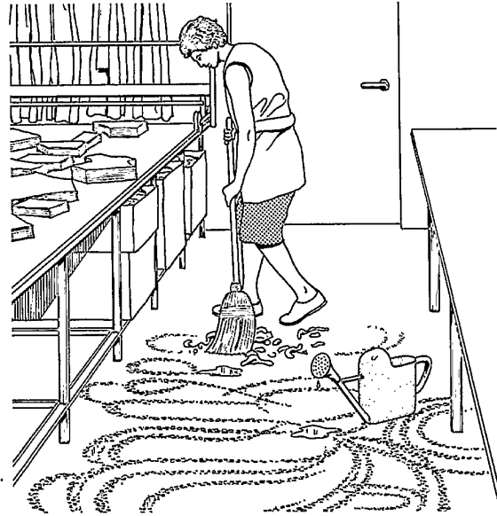
Figure 5: It is good practice to clean the floor at least once a day. Spraying water on the floor before brushing prevents spreading dust
