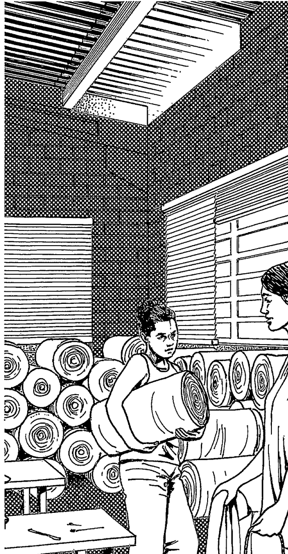
Figure 10: In hot tropical countries walls provided with special bricks and pre-cast concrete panels with fixed louvres improve the intake of fresh air
